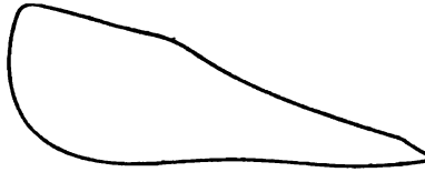
Fig. 255. Indicator Card with Steam Lap too large.
